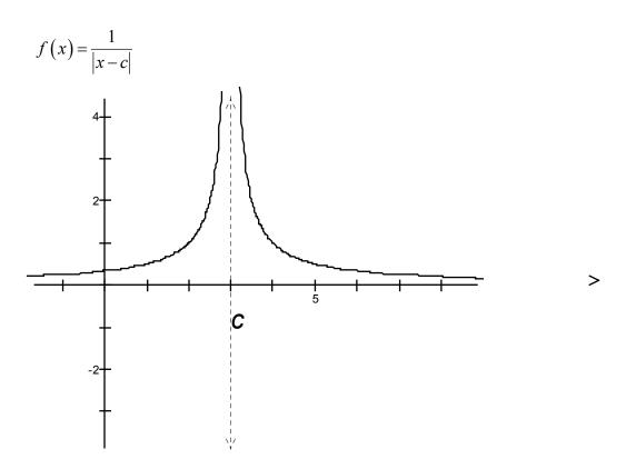
Here f(x) increases from both directions, however it does not approach a finite value.
